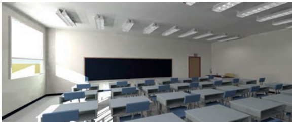
Installing Solera ® above the vision glass units dramatically cuts back glare, converting it to soft, well-distributed diffuse daylight.
